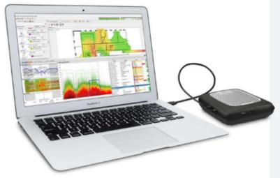
The ESS™ Pro software is an easy-to-use application and allows you to design Wi-Fi networks automatically indicating the optimal location and configuration of access points. Also ESS™ Pro makes it possible to perform quick and easy site surveys, analysis, optimization and troubleshooting in existing Wi-Fi networks.
